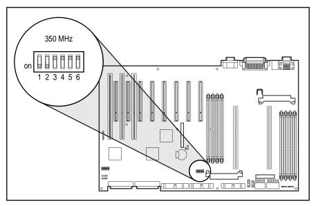
Figure 4-4. 350 MHz processor switch location and default setting
